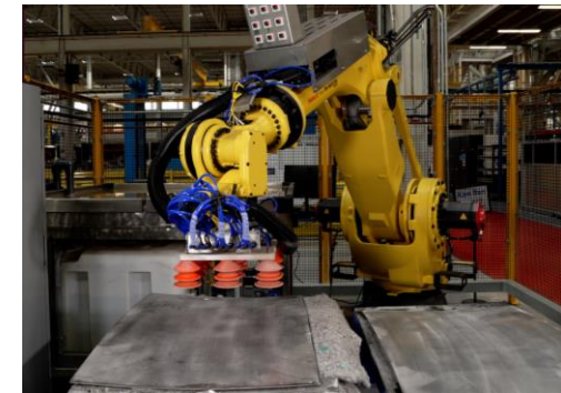
Ultrasonic inspection system on transition panels
