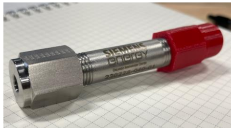
Water detection sensor developed, manufactured, and tested by TAC team.
