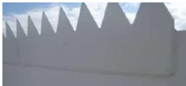
Figure 2: Blade with DinoTails or serrations
