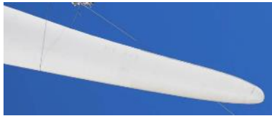
Figure 1: Blade without DinoTails or serrations
