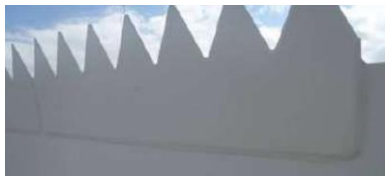
Figure 2: Blade with DinoTails or serrations
