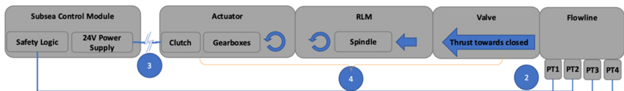
Fig. 1. eHIPPS system design overview
