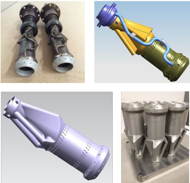
Figure 19: Fuel burner design progressions from welded (top left) to SLM additive manufacturing (bottom right) for 3rd generation DLE burner.
