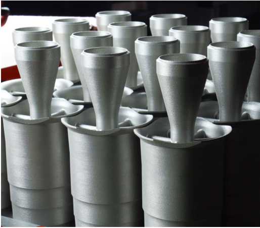
Figure 18: Additive manufactured premixed combustion swirlers for heavy-duty large gas turbines.
