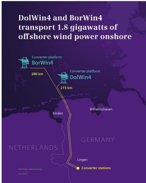
Two new power links set the course for more wind energy in the German power grid: **DolWin4 and BorWin4 will transport up to 1.8 gigawatts** of green wind power from several wind farms in the German North Sea to land with low losses.
