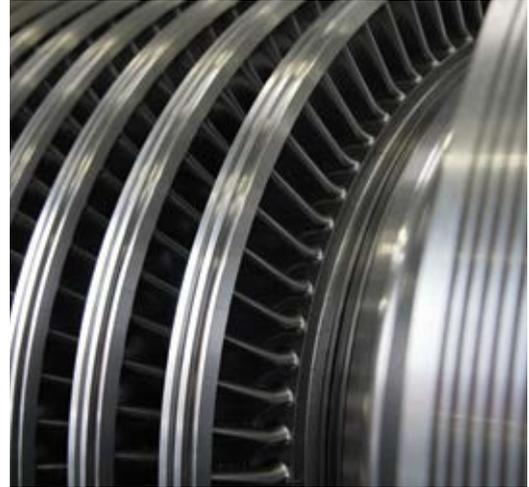
Fig. 2: Reaction stage
