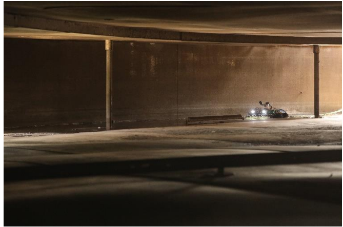
Figure 1 Remotely operated TOKA™ inspects tank floor.
