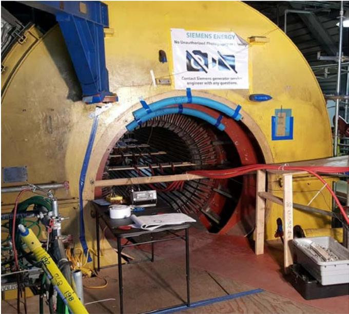
*Figure 8: Elevated Frequency Loop Test Setup*
