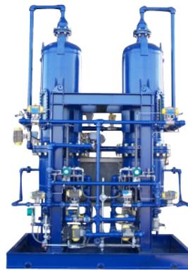
The filter operates at twice the flux rate of conventional sand filters in the same application, and can remove over three times the amount of solids before needing to be cleaned.
