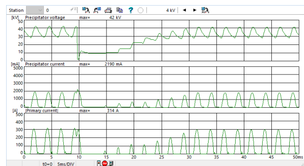
SIPREC oscilloscope: signals for secondary voltage / secondary current / rectified primary current at flashover processing
