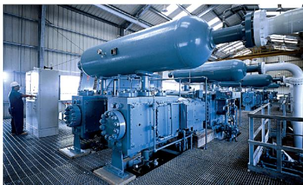
**Figure 1.** A Siemens Energy reciprocating compressor in operation.
