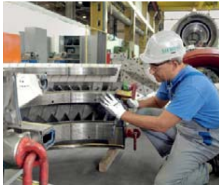
Blading of turbine rows
