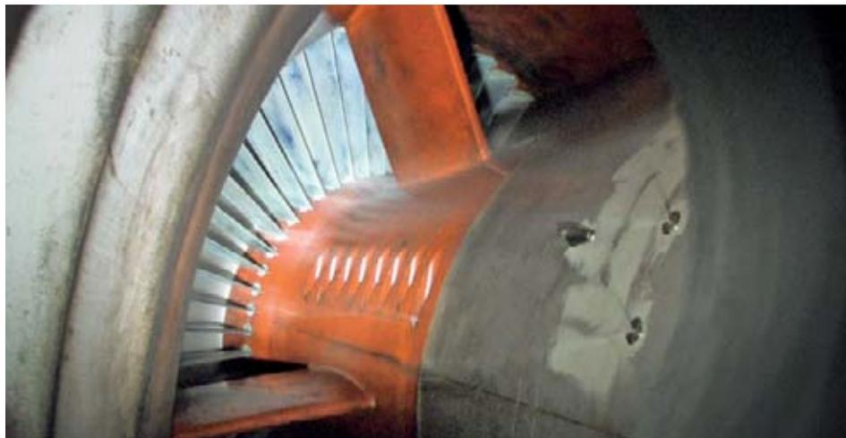
Air intake inner cone with nozzles – on-line washing
