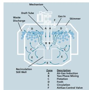
The Quadricell® separator uses four cells in series for maximum liquid/air contact. Cells are individually adjustable for maximum skimming efficiency and optimum air introduction for any set of conditions. The separator is designed to provide high performance and greater throughput capacity for the
