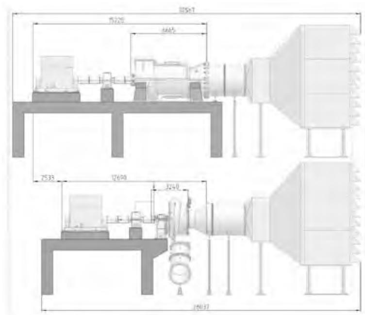
**Figure 2.** Train length comparison with axial (top) vs integrally geared compressor (bottom).
