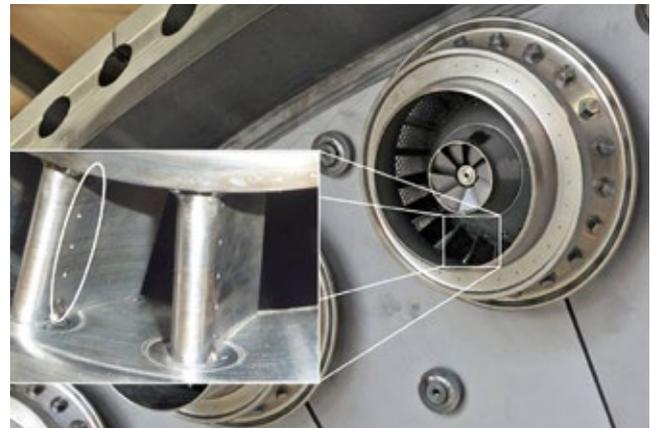
Fig. 3: A closer look at required hardware design changes for the modification of fuel gas quality
