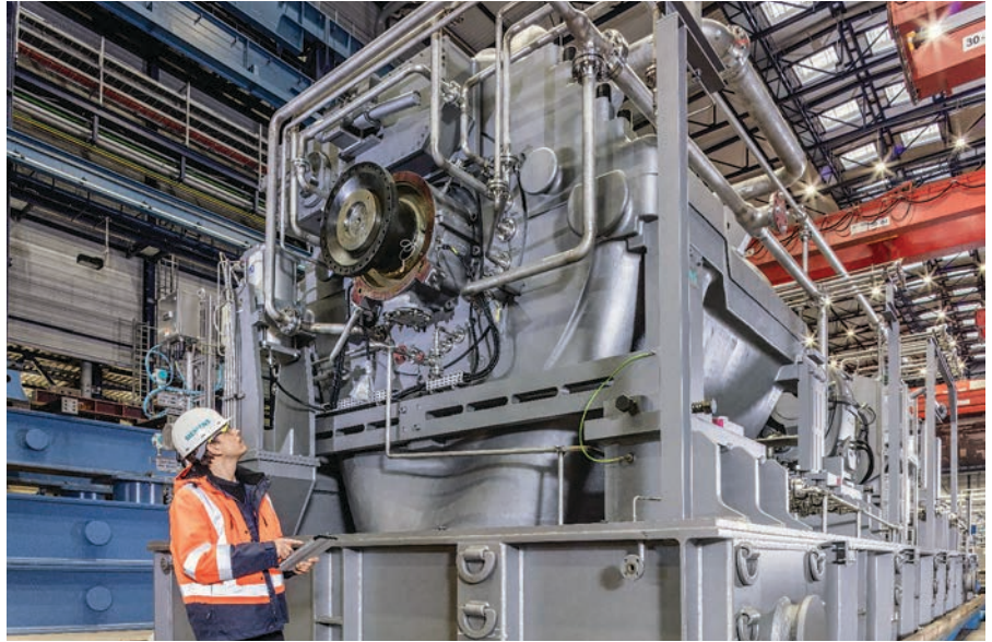
FIG. 4. LNG compressors are available for the following services: Main refrigeration, boiloff gas, end-flash gas, natural gas booster and recycle compressors.
