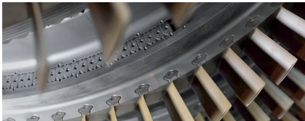
Optimized compressor blades and vanes
