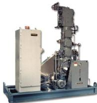
Whether direct-connected or belt-driven, the ESH can handle a variety of drivers up to 70 hp (52 kW) and can be fitted with either lubricated or non-lubricated cylinders from 1.625 to 19 inches (41 to 483 mm) in bore diameter. The ESH is also available in a vertical arrangement that greatly reduces the foundation size and area. In its vertical configuration, the "ESV" provides significant advantage where space may be limited.
