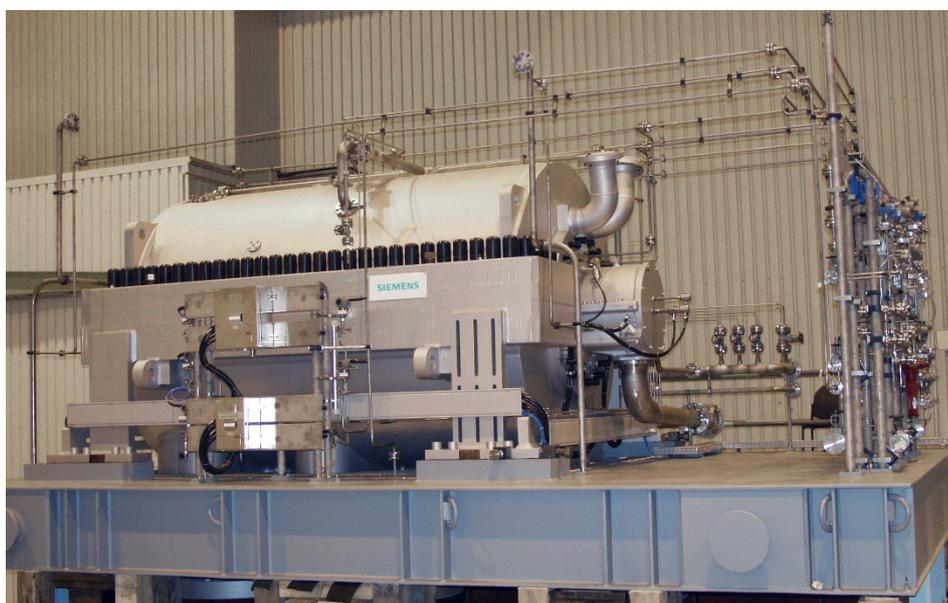
**Above:** STC-SH propylene turbo compressor for an ethylene plant.
