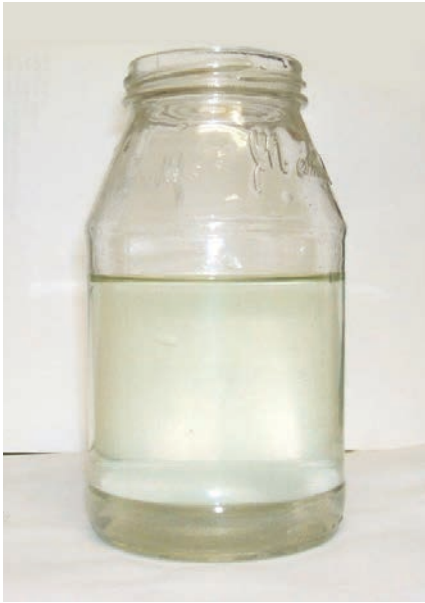
Landfill leachate is shown after it has gone through treatment. Siemens Energy, Inc.
