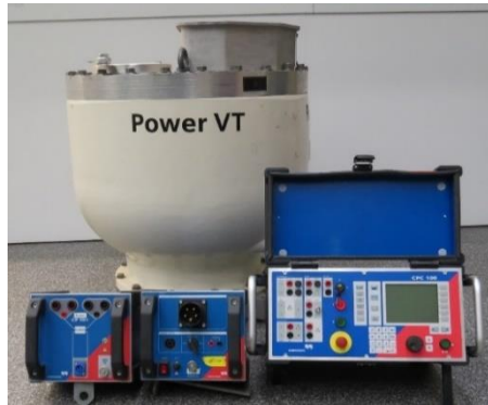
Power VT high-voltage test set-up
