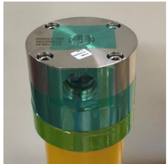
MK-II adapter installed, and sealing tape applied
