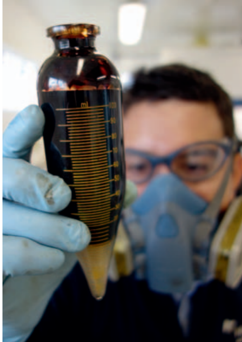
A chemist examines a sample of heavy oil to analyze how effective the water dehydration process has been.
