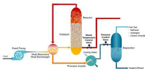
**Figure 2.** Catalytic gasification technology process flow diagram.
