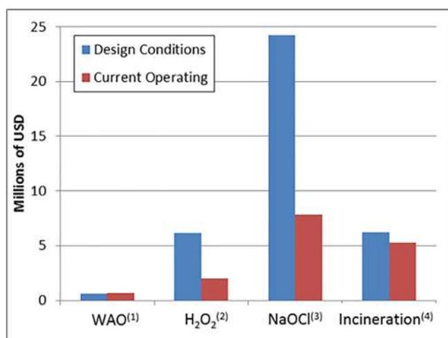
**Figure 1.** Comparison of annual operational expenses between WAO technology vs traditional oxidation treatment alternatives for treating ethylene spent caustic at current operating conditions and design conditions. (1) Includes electricity, steam, boiler feedwater, cooling water, and instrument air; (2) H<sub>2</sub>O<sub>2</sub> only; (3) NaOCl only; (4) fuel only.
