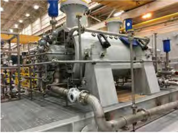
**Figure 3.** A typical Siemens Energy hydrogen recycle centrifugal compressor package.
