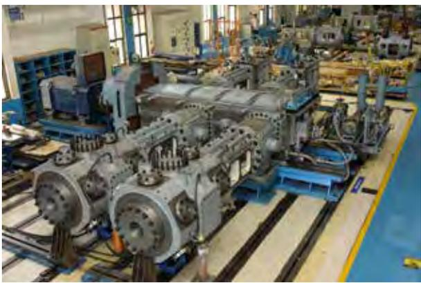
**Figure 2.** HHE-VL compressor, 4 throws, hydrogen application on test stand in the Naroda, India facility; shipped in 2020.
