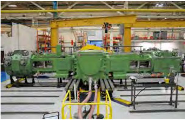
**Figure 1.** BDC-18H3 compressor, 4 throws, hydrogen application, 3,000 psia discharge pressure; shipped in 2019.
