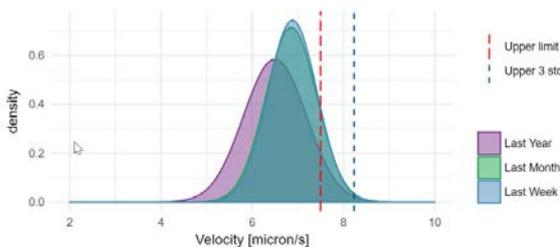
**Figure 5.** Deviations and tendencies of vibration levels of a pump as one asset health KPI.
