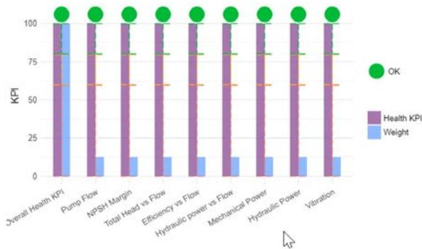
**Figure 3.** Asset health can be visualised on web-based dashboards based on KPIs for condition-based performance monitoring of specific WWTP assets.
