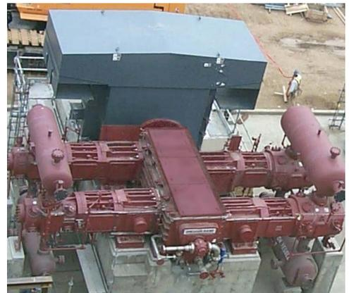
Rugged, precision-machined tri-metal main and crankpin bearings are generously sized for long-lasting service. Bearings are positioned on both sides of each pair of crankthrows. All bearings are forced-lubricated per API-618 specifications. Connecting rods are rifle-drilled for lubrication of the crosshead pin bushing.
