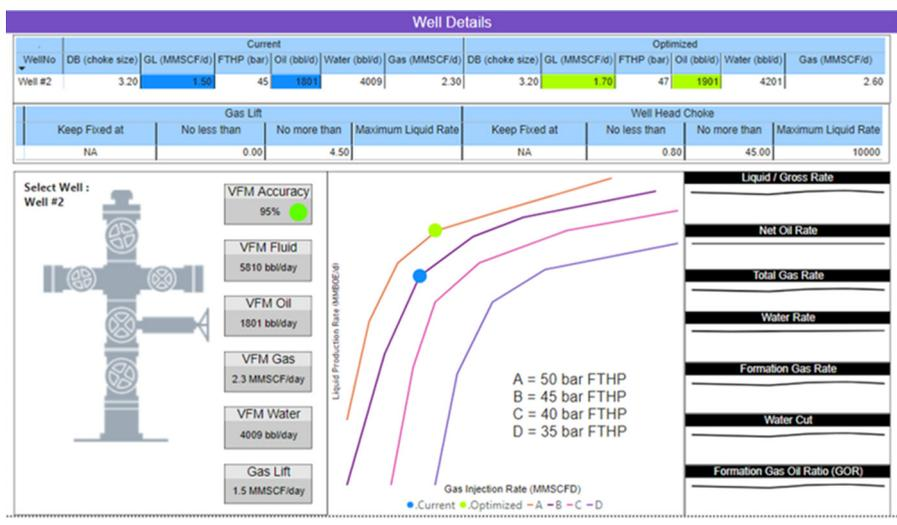
form (delivered as a service), enabling rapid modeling and optimization of the entire upstream value chain—from the sand face through central processing facilities to the sale of the product, Fig. 1. It differs from conventional sequential modeling tools, in that it uses an equation-based optimization engine from Siemens Process Systems Enterprise, known as gPROMS Oilfield.
