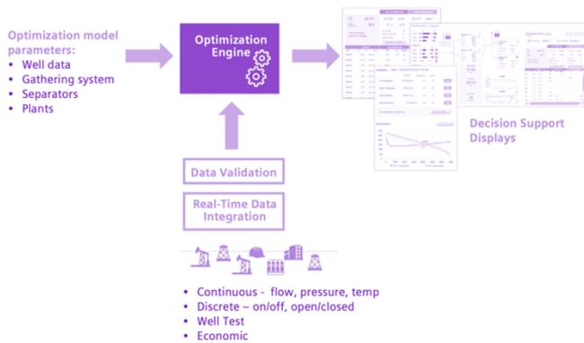
Figure 1: Overview of RTPO workflow
