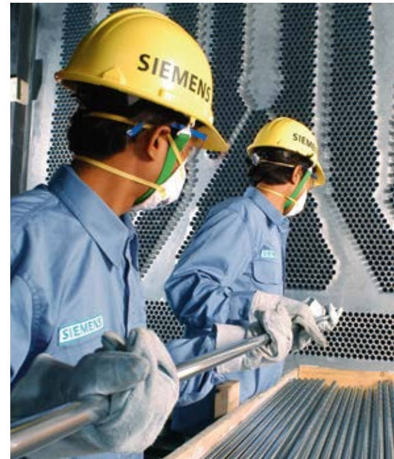
Tubing of the new Farge condenser at the Siemens manufacturing plant
