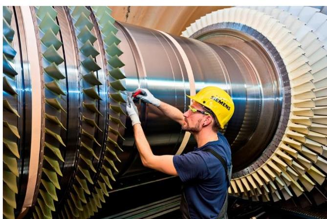
Pictured: Siemens SGT5-4000F gas turbine
