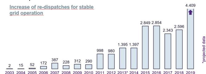
Fig. 1: Increase of re-dispatches from TSO for frequency and voltage stabilization caused by an increase of renewables and reduction of stabilizing, syn-chronous generation technologies in Tennet-Zone, Germany
