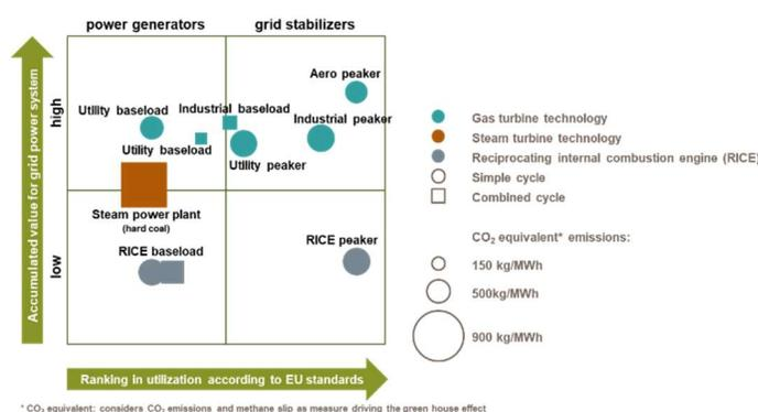
Fig. 5: Qualitative comparison of generation technologies considering the ranking within the merit order positions according to (EU) 2017/2195 [4] for the several grid services versus the overall benefit considering **all grid services** as described in (EU). Grid services mean support of generation, grid balancing for frequency, voltage, and short circuit power as well as grid restoration capabilities.
