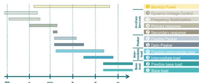
Fig. 3: Operating pattern based power market segmentation [Siemens].
