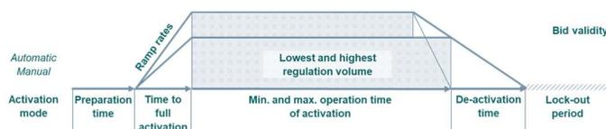
Fig. 4: Overview about the evaluation criteria for Merit Order lists per grid service according to (EU) 2017/2195.
