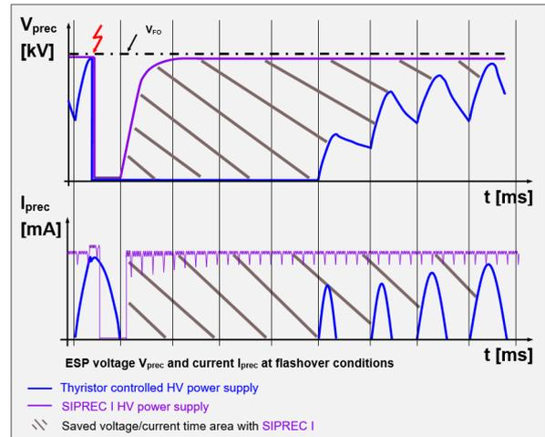
Flashover / sparks must be detected immediately and the short-circuit currents feeding the arc must be stopped as quick as possible to keep the ESP voltage and current values or to enable the fast recovery.
