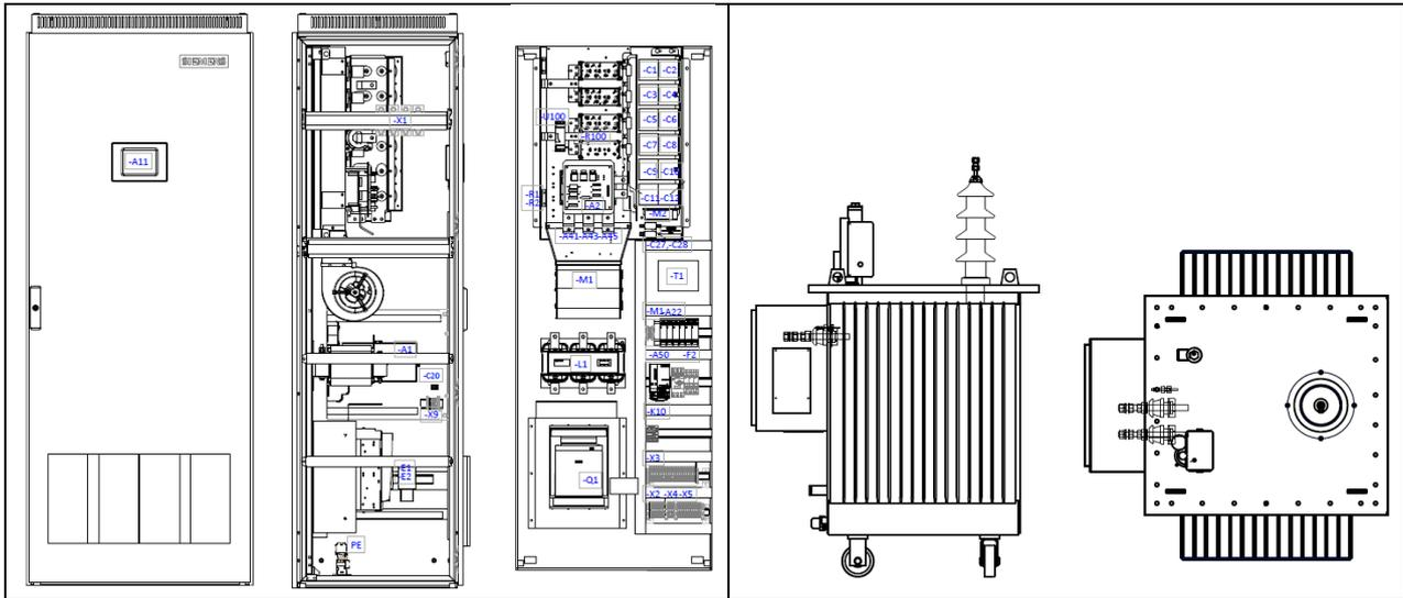
For new ESP installations we recommend installing the SIPREC I power supply system consisting of the SIPREC I control cubicle and the SIPREC TR500 T/R set for maximum performance. For retrofitting of existing ESPs, we also offer SIPREC I Hybrid IGBT control cubicle for the reuse of existing and suitable 50Hz/60Hz T/R sets.
