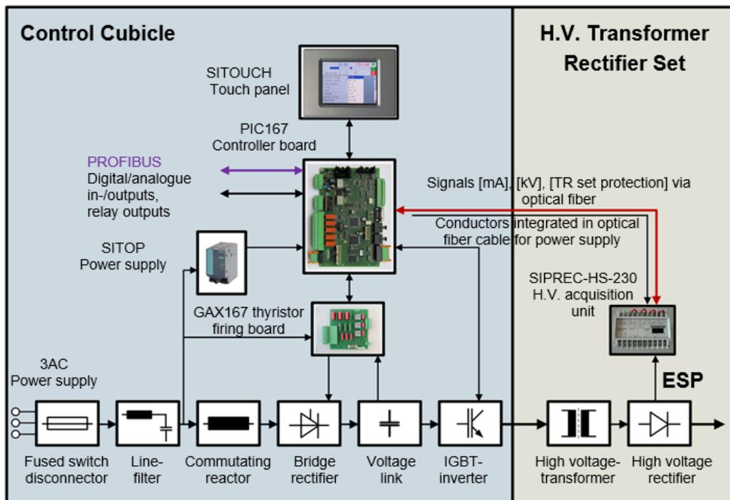
The SIPREC I control cubicle consists of a fuse-switch-disconnector with semiconductor fuses, a line filter, the commutation reactor, a half-controlled six-pulse bridge rectifier, the voltage link capacitors, the IGBT power semiconductor modules and SIPREC controller components. The controlled rectifier charges the voltage link and is operated like an uncontrolled diode bridge when a certain link voltage
